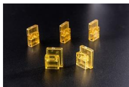
Lens array for optical module
