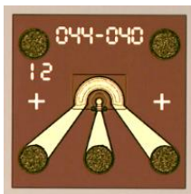
56Gbaud PIN Photodiode Chip
